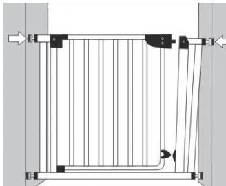
› The gate must be fixed to a solid and suitable surface. Do not fix it between windows openings or similar. Incorrect fitting or positioning can be dangerous.
